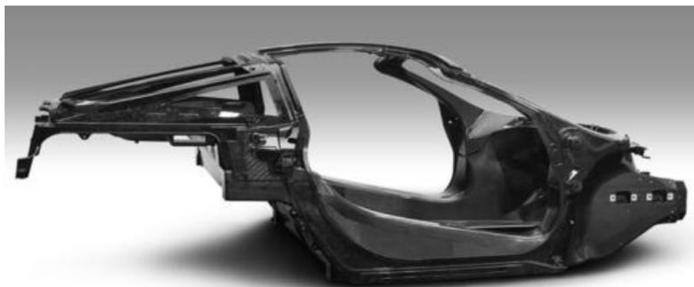
**Gambar 18.** Chassis mclaren carbon (AutoNetmagz, 2017)
