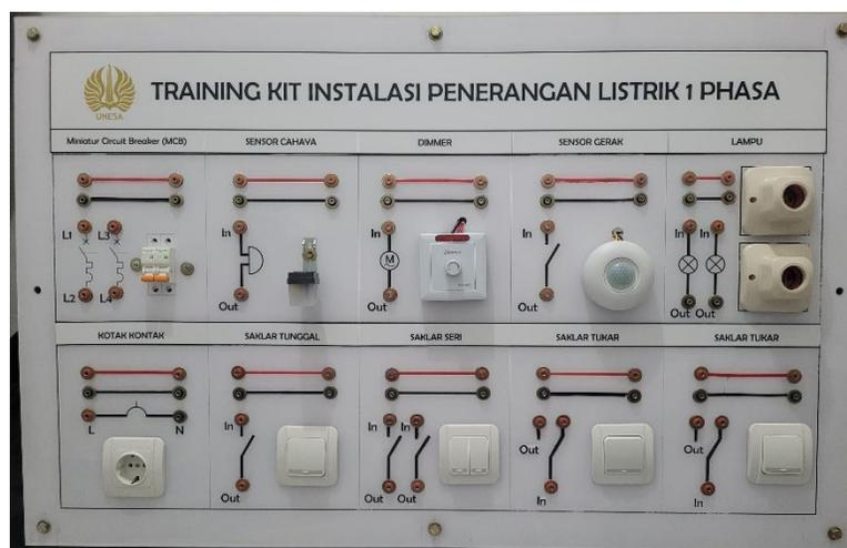
Gambar 3. 2 Taining Kit Instalasi penerangan Listrik 1 Phasa
